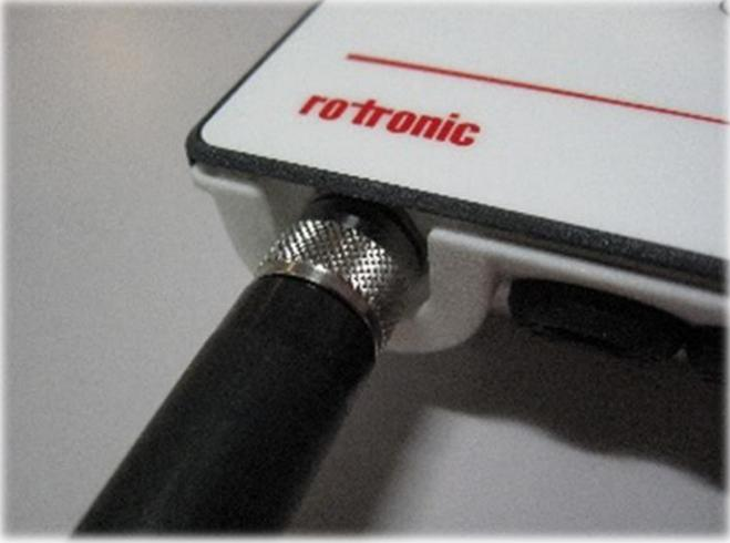
A close-up photograph showing a black probe with a silver knurled metal connector being inserted into a white plastic port on a device. The device has the 'rotronic' logo printed in red on its top surface. A thumb screw is visible on the side of the port, used to secure the probe. |
