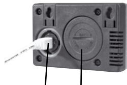
USB Mini-port (settings and data download) Battery compartment (BAT.)
